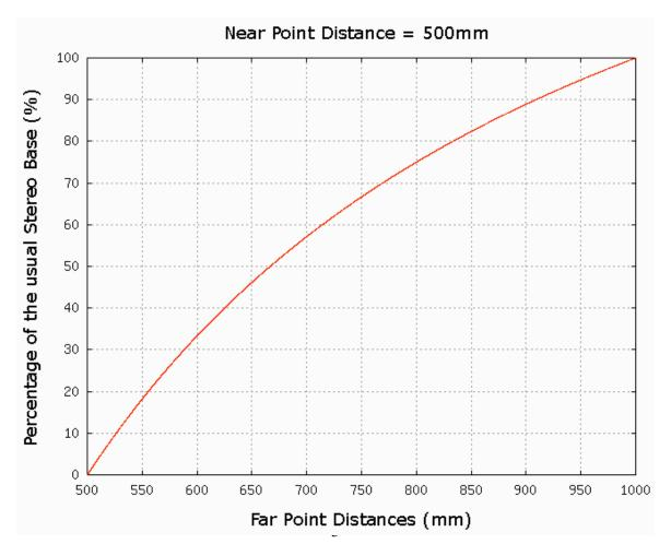
Not only does this deliberate tapering of the stereo base avoid exaggerated depth and allow a proper depth rendition in shallow subjects, but it also permits a trivial calculation for the stereo base.
